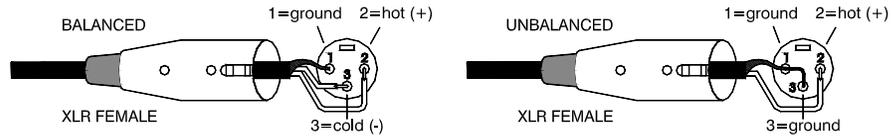
Differentially balanced, low impedance line level outputs are provided on XLR. These are capable of driving long cable runs to the amplifier racks without loss or interference pickup. Use balanced connections wherever possible. To drive unbalanced equipment inputs wire the plug as shown on the right. Use high grade shielded cables for audio connections.
