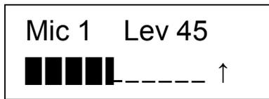
**Level Up** Here, the function key has been assigned to increment the level of the associated input, output channel or matrix crosspoint when pressed. Each press increases the level and the displayed bar by a value of 5. Holding down the key automatically scrolls the value up. A minimum and/or maximum value may be assigned.
