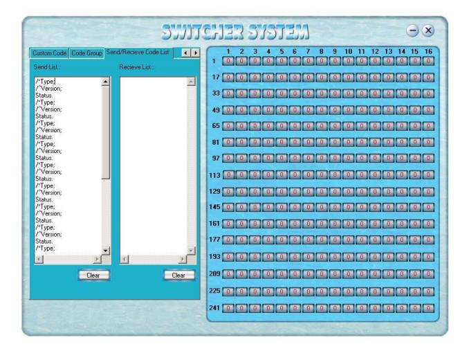
Send List window: Lists sent command code Received List window: Lists feedback from the switcher Clear: Clears either of the two lists
