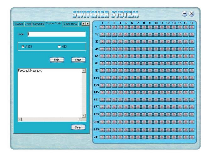
Select between ASCII and HEX format command codes (for command details, please refer to section) Help: Displays the list of commans codes.
