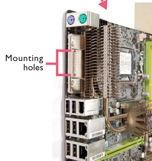
Internal view of the chassis (rear I/O area)
