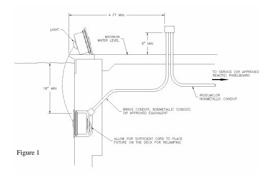
Install fixture in a vertical pool or spa wall – not in floor. Failure to install the fixture properly could result in personal injury and/or property damage.
