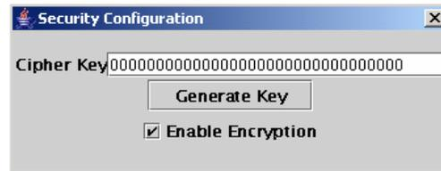
**NOTE:** The modem must be set to Gateway mode for the encryption feature to work regardless of whether it is enabled on this menu.
