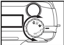
**1 Rotate the function dial to "SETUP" and slide the power switch to turn on the camera.**
