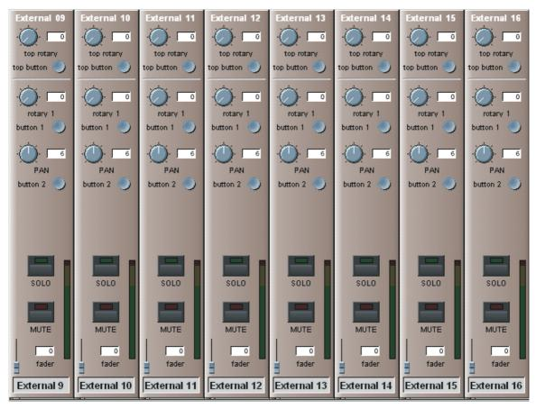
MIDI Messages are defined by touching the relevant on screen control and entering a MIDI channel, a command type and values for the parameters. At the bottom of the panel a MIDI port can be selected - Port A represents the first COMBI card, B is the second COMBI card and T is the standard built in MIDI port on the console.
