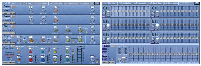
**Graphics EQ's** can be ganged with relative offsets by pressing the relevant on screen **Gang** buttons and individual faders can be reset using the worksurface master solo buttons.
