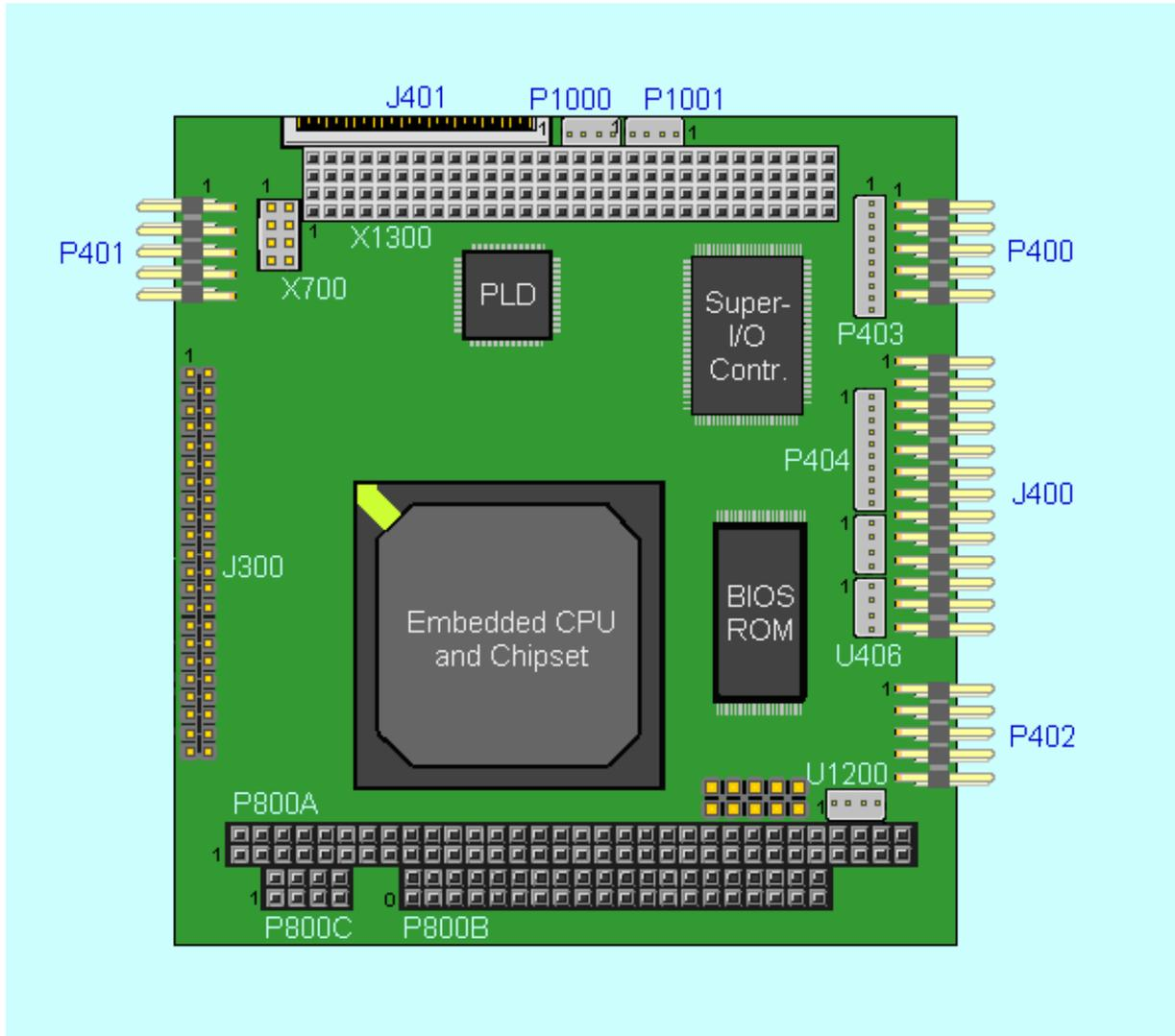
Pin 1 of any connector is marked with “1” in this drawing and with a rectangular pad at the bottom side of the board’s PCB.
