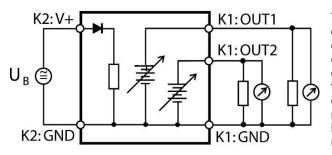
The maximum permissible cable length can be determined under consideration of the voltage drop caused by the current flowing to the devices connected to the unit. The voltage drop in the cable depends both on cable resistance and on the equivalent resistance of the devices connected in parallel to the unit. The total resistance connected to each unit output should be at least 1000 ohms. Cable resistance should not be more than 1/1000 of the load resistance.
