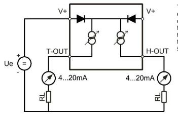
The maximum permissible cable length connecting the HF32 to other devices is determined by the total resistance resulting from the addition of the cable resistance and that of the devices connected in series with the unit. This resistance should not exceed 500 ohms.
