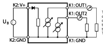
The maximum permissible cable length, connecting the unit to other devices, is determined by the total resistance resulting from the addition of the cable resistance and that of the devices connected in series with the unit. This resistance should not exceed 500 ohms.
