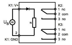
NC: normally closed contact (relay not energized)
