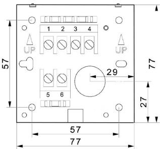
Type R and type S consist of a base plate and an electronics module that plugs into the base plate. The base plate is installed and wired first.
