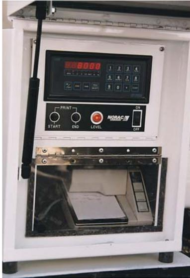
Indicator, OnBoard Circuit Board and Printer are all housed in the Weigh Center.
