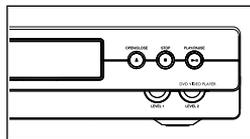
→ To adjust the volume of microphone, turn the knob LEVEL1 or LEVEL2 on the right of front panel.
