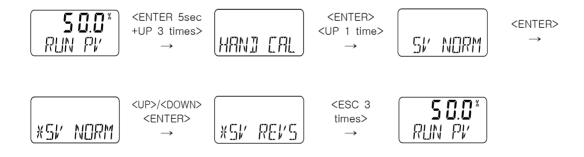
Positioner's PV values can be same or reversely output with the actual stroke. EX ) NORM Mode current 0% shall be converted into 100% in case of REV.
