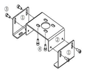
Figure 3-9: Bracket set for rotary positioner installation
