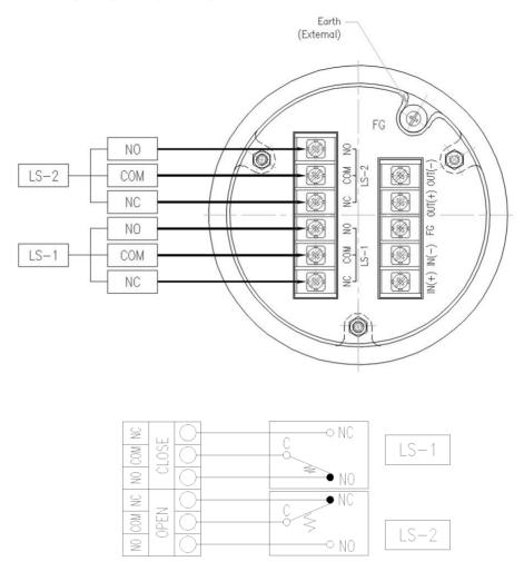
Figure 5-3: Limit switch connection map
