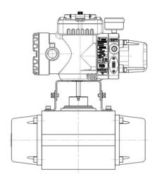
Figure 3-7: Namur type installation
