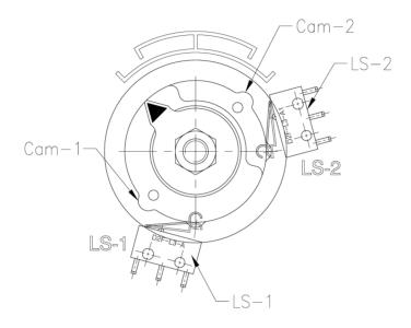
Figure 6-1: Adjustment of limit switch operation
