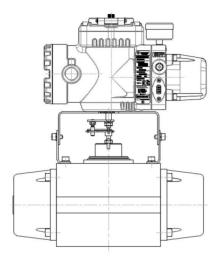
Figure 3-7: Fork Lever type installation
