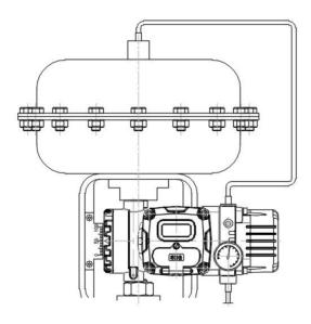
Figure 4-1 Single acting linear actuator
