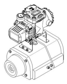
Figure 4-2: Single acting rotary actuator
