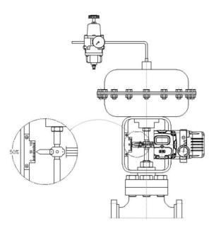
Figure 3-3: SP760 positioner installation in actuator
