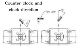
② With an actuator's initial start point of 0%, install the fork lever as seen in figure according to the rotation direction of stem. Make sure the installation degrees of fork lever should be 45 degree from the horizontal line.
