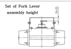
③ If fork lever position is set, tighten the nuts, which is assembled with the lower parts of fork lever to an actuator stem firmly. At the moment, the fork lever upper side and the upper bracket's distance should be 19 to 25 mm each other.
