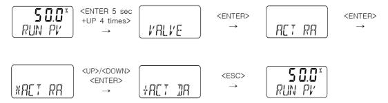
\* This work must be done after shut down air or 50% position condition. In this time ,actuator shall be operated reversely .
