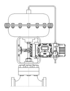
Figure 3-1 : SP760 Installation example
