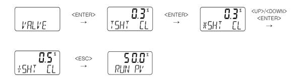
Set according to the connection method of single actuator and positioner. Ex )The above 8 standard lever type and adapter lever type is LEV setting while adaptor lever type and rotary type are STD setting.
