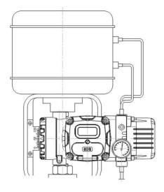
Figure 4-3 Double acting type linear actuator
