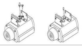
4 Attach the positioner onto upper bracket and fix it with bolts. At this moment, insert the pin on the lower part of the fork lever into the hole of fork lever so that it may be centered. When tightening bolts, do not connect one bolt firmly and after loosing 4 pcs of bolt slightly and
