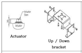
① Connect up/down bracket assembles onto an actuator with bolts. Note the positioner manufacturer doses not supply bolts to fix an actuator.
