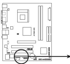
FLOPPY1 PIN 1 NOTE: Orient the red markings on the floppy ribbon cable to PIN 1.
