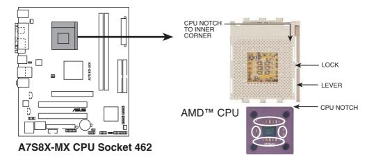
2. Unlock the socket by pressing the lever sideways, then lift it up to a 90°-100° angle.
