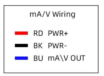
※Note: When wiring, connect the positive and negative poles
