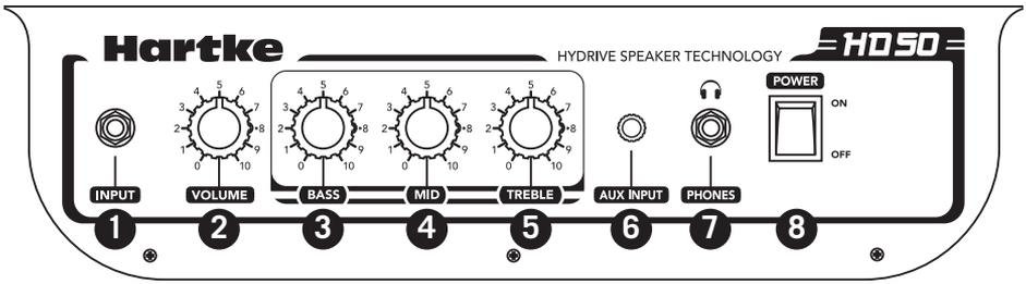
1. **INPUT** - Connect your bass guitar here using a standard  $\frac{1}{4}$ " unbalanced instrument cable.
