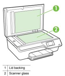
⚠ CAUTION: Use only glass cleaner to clean the scanner glass. Avoid cleaners that contain abrasives, acetone, benzene, and carbon tetrachloride, all of which can damage the scanner glass. Avoid isopropyl alcohol because it can leave streaks on the glass.
