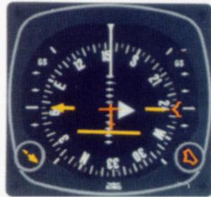
2. Halfway through the outbound turn, the KI 525A display shows the Deviation Bar behind the symbolic aircraft. You know, therefore, that you must eventually fly back to the radial in order to be on course during the inbound leg of the holding pattern.
