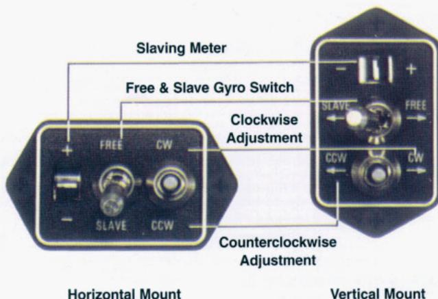
**Slaving Meter** — This meter indicates the difference between the displayed heading and the magnetic heading. Right deflection indicates a clockwise error of the compass card. Left deflection indicates a counterclockwise error of the compass card. Whenever the aircraft is in a turn and the card rotates, this meter will show a full deflection to one side or the other.
