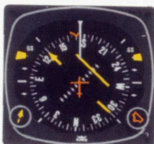
2. Capturing the ILS course can be accomplished without overshooting or bracketing with the same technique you used in intercepting an enroute course: simply keep the top of the Deviation Bar on the Lubber Line and coordinate your turn until the bottom of the bar is aligned with the Course Arrow. Each dot on the LOC Deviation Scale represents 1/2° deviation when tuned to an ILS frequency.
