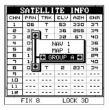
the desired group letter is showing in the box (and in the background), press the up arrow key to change it. A screen similar to the one at right appears.
