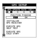
If you wish to turn the position pinning feature on, press the MENU key, then highlight the "GPS Setup" label and press the right arrow key. Now highlight the "Position Pinning" label. Finally, press the right arrow key.
