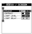
To turn the speaker off, highlight the "SPEAKER" label on the "Audio/ Screen" menu and press the right arrow key. Now press the left arrow key to turn the speaker off. Repeat these steps to turn the speaker on. Press the EXIT key to erase this menu.
