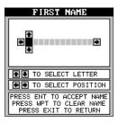
process until the I.D. is complete. You can press the WPT key to completely erase all of the characters you entered and start over, if you need to. Pressing the EXIT key erases this screen without accepting any input. When the first name is correct, press the ENT key.
