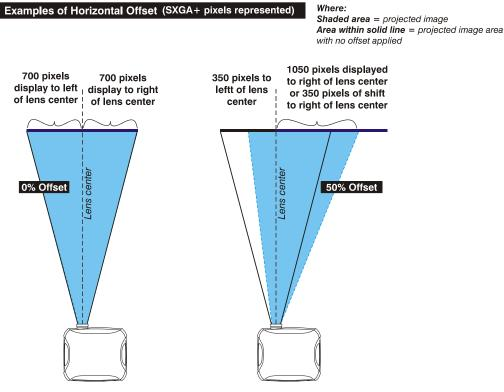
**#1** In this example, no offset is applied. Therefore half of the image appears to the left or lens center and half appears to the right.
