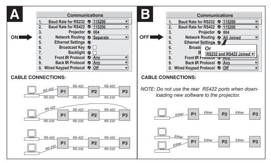
Figure 3.8. Using the "Network Routing" Option
