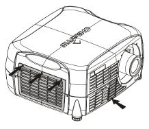
Figure 4.6. Remove Filter Access Panels
