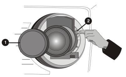
Figure 4.9. Depressing Lens Release
