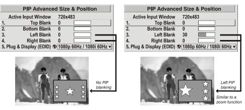
Figure 3.6. Blanking of a PIP Image
