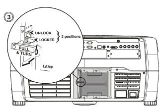
Figure 4.3. Release the Lamp Lock
