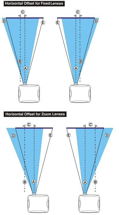
Figure 2.4. Lens Horizontal Offsets
