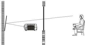
Figure 2.5. Folded Optical Path
