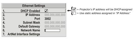
Figure 2.15. Setting the Projector's IP Address
