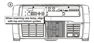
Figure 4.5. Insert New Lamp Module
