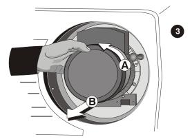
NOTE: Connector assembly will move as you turn the lens.
