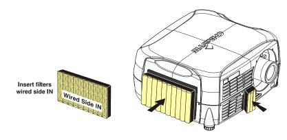
Figure 4.7. Insert New Filters
