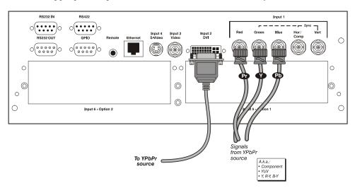
Figure 2.8. Connecting YPbPr sources
