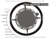
Figure 4.11. Adjustable Screws on Retaining Ring
