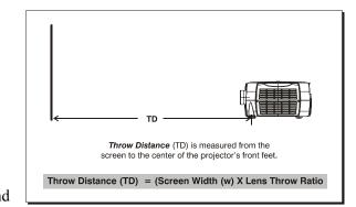
**NOTES: 1)** Throw distance is measured from the screen to the center of the projector's front feet. **2)** This measurement is not necessarily parallel to the floor as the projector and screen may be inclined. **3)** Due to lens manufacturing, throw distance calculations have a tolerance of  $\pm 5\%$ .
