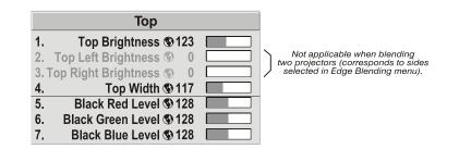
6. The brightness and black hues of the blended region can be adjusted in more detail in case fine-tuning is needed (may be only necessary for blending a 2 x 2 projector display because of blending differs for the sides and center).
