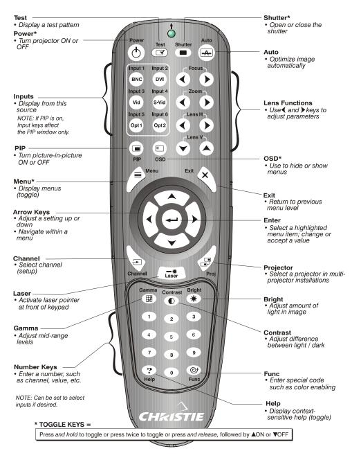
\*These are toggle keys, which require you to press and hold or press twice or press and use the up/down arrow keys.
