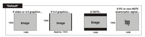
• Select "NO RESIZING" to display the image in its native resolution, which may or may not match the projector's resolution. For example, for a source with a native resolution of 800 x 600, "No Resizing" in an SXGA+ projector will use the central 800 x 600 pixels and have a black border—the black border areas are unused areas. See below.
