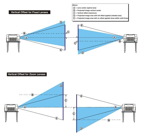
Figure 2.2. Lens Vertical Offsets
