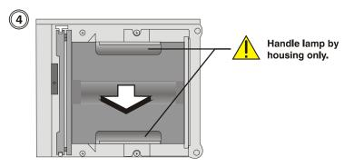
Figure 4.4. Remove Lamp Module
