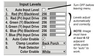
monitoring image content and adjusting the controls appropriately—further adjustment is typically not required to obtain proper blacks or whites.
