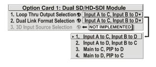
slots is empty, the corresponding read-only menu entry does nothing. If there is a module installed, the corresponding menu entry may activate a submenu of further options pertaining to that module.
