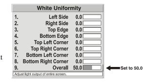
exceed **50.0** for "Overall"—a higher level will likely interfere with achieving brightness uniformity and is not recommended.
