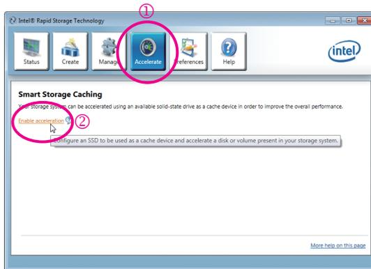
(Note 1) The SSD works as a cache of the hard disk. The maximum cache memory size is 64 GB. If you use an SSD larger than 64 GB, the space beyond 64 GB can still be used for storing your data.
