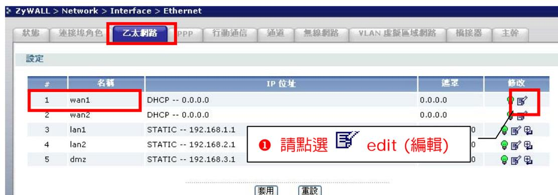
The screenshot shows the ZyWALL configuration interface for Ethernet. A table lists interfaces: wan1 (DHCP), wan2 (DHCP), lan1 (STATIC), lan2 (STATIC), and dmz (STATIC). A red box highlights the 'wan1' row, and another red box highlights the 'edit' icon in the '修改' column. A callout box with a red '1' says '請點選
