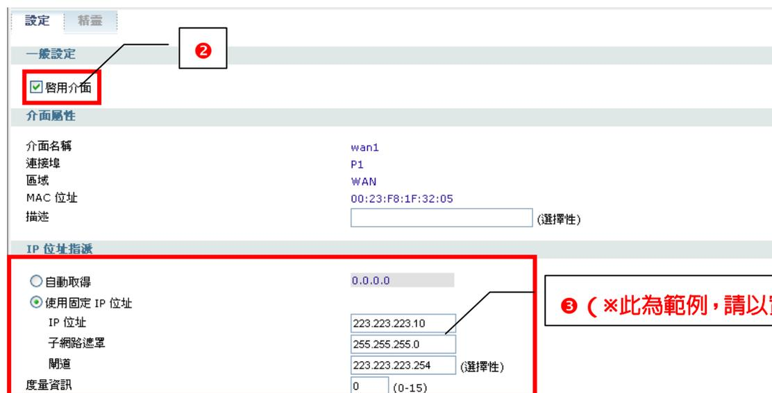
The screenshot shows the configuration page for the 'wan1' interface. A red box highlights the '啟用介面' checkbox, with a callout box containing a red '2'. Another red box highlights the '使用固定 IP 位址' radio button and the input fields for IP address (223.223.223.10), subnet mask (255.255.255.0), and gateway (223.223.223.254), with a callout box containing a red '3' and the text '(\*此為範例，請以實際資訊輸入)'.
