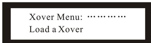
Press <NEXT> or <BACK> button, you can navigate forward or backward the Xover submenus: Load a Xover, Design a Xover, Store a Xover and Erase a Xover. Confirm by pressing <ENTER> button.
