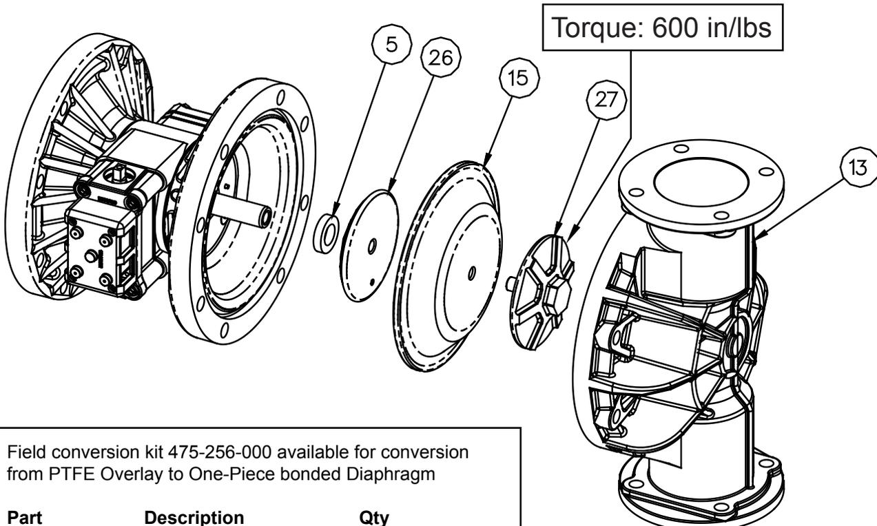
Field conversion kit 475-256-000 available for conversion from PTFE Overlay to One-Piece bonded Diaphragm
