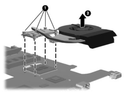
NOTE: The following illustration shows the fan/heat sink assembly removal process on a computer model equipped with an Intel processor, the Intel HM45 chipset, and a graphics subsystem with UMA memory.
