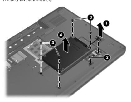
8. If it is necessary to replace the hard drive connector cable (1), the hard drive screws (2), or the hard drive bracket (3), remove and replace the components.
