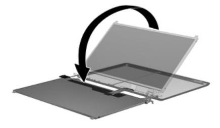
Release the adhesive strip (1) that secures the display panel cable to the display panel, and then disconnect the display panel cable (2) from the display panel.
