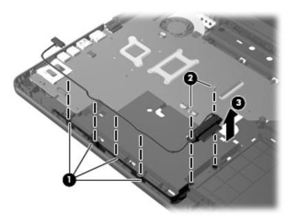
Reverse this procedure to install the optical drive connector cable.
