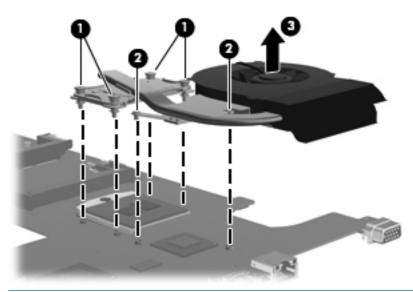
NOTE: The following illustration shows the fan/heat sink assembly removal process on a computer model equipped with an Intel processor, the Intel HM65 or HM55 chipset, and a graphics subsystem with UMA memory.
