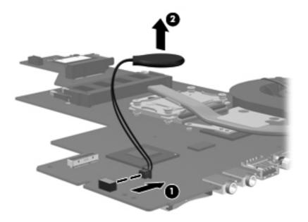
Remove the RTC battery.
