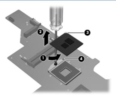
Reverse this procedure to install the processor.
