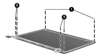
**b.** Lift the top edge of the display panel, and then swing it up and forward until it rests upside down in front of the display enclosure.
