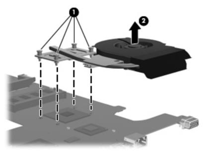
NOTE: The following illustration shows the fan/heat sink assembly removal process on a computer model equipped with an Intel processor, the Intel HM65 or HM55 chipset, and a graphics subsystem with discrete memory.
