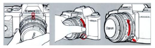
To mount the lens, first align the red positioning point on the lens with the red dot above the camera mount as illustrated.
