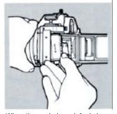
When the rewind crank feels loose, open the back cover. The frame counter will automatically return to "S." Remove the film cartridge as illustrated and place it back in its canister. It should be developed as soon as possible.
