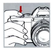
Press the shutter button all the way. The film will automatically advance to the next frame.
