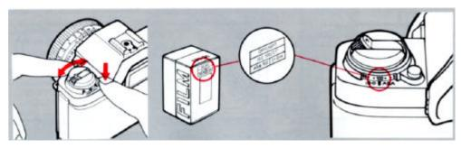
While pressing the lock release button, rotate the film speed dial until the ISO/ASA of your film is aligned with the green index. This is necessary for getting correct exposure.
