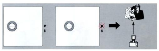
Depress the shutter button halfway; once the "!" mark signals that the flash is charged, you are ready for flash photography.
