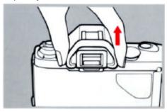
Ten eyesight correction lenses are available in the powers of +3, +2, +1.5, +1, +0.5, 0, -0.5, -2, -3 and -4 diopters. They may make viewing and focusing easier if you are near- or farsighted. Slide the Eyecup T up to remove it before you attach the dioptric adjustment lens to the camera. Choose the one which is closest to your eyeglass prescription, and make a practical test if possible.
