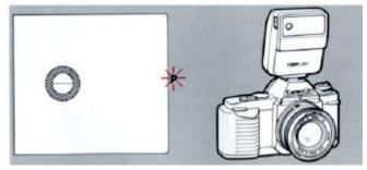
Switch to flash photography when the green "P" starts to blink. For best results, we recommend using the 244T with the T50. It is incredibly easy to use, and has been designed exclusively to go along with the T50.
