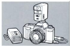
This accessory is a remote control photography device using infrared rays to control cameras from a distance. The LC-1 is particularly useful in sports photography, wildlife photography, news coverage, and for numerous other fields. The Wireless Controller LC-1 consists of a transmitter and a receiver. Up to three cameras can be operated in series when the receivers are set to different channels
