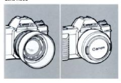
We strongly recommend the use of a lens hood to keep out side light which may cause flare and ghost images to form on the image. Rigid Canon hoods also help to protect the lens from shock. Use only a hood which is specified for your particular lens. Most Canon hoods fit into the bayonet mount and are fixed by turning. For more details, please see the lens instruction manual.
