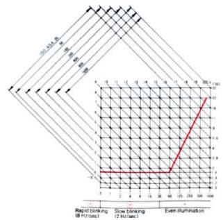
The solid line indicates the meter coupling range in programmed AE when the FD 50 mm f/1.4 is used.
