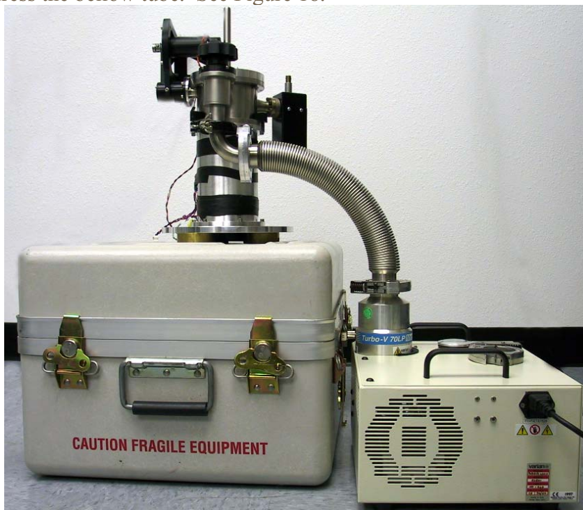
Figure 18. Turbo pump connected to dropping chamber. Note the minimum stress in the hose.
