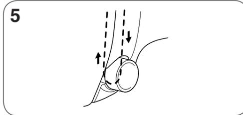
5 Pass the thread into the thread tension discs or behind the thread tension dial from the right to the left.
