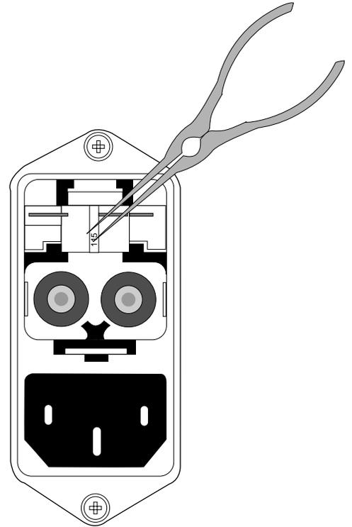
**3:** Use a small pair of needle-nose pliers to gently pull out the mains jumper.
