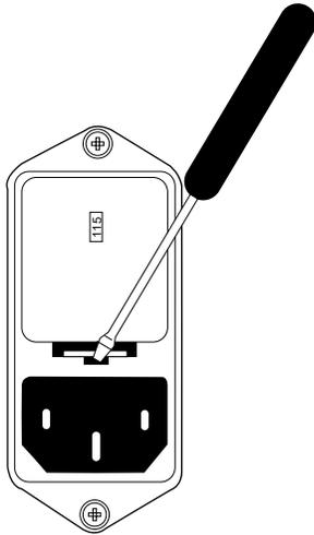
**1:** Insert a small screwdriver into the slot beneath the fuse sled and gently press in and up. The fuse sled will pop out approximately 3/8" inch.
