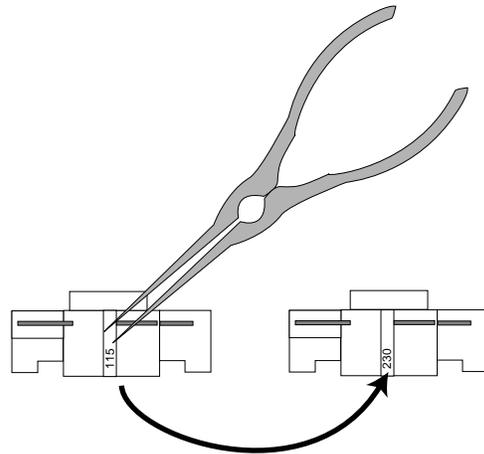
**4:** Use the needle-nose pliers to reverse the mains jumper so that the other voltage value is facing outwards, then reinsert the mains jumper. Finally, reinsert the fuse sled by gently pushing it back in until you hear a click.
