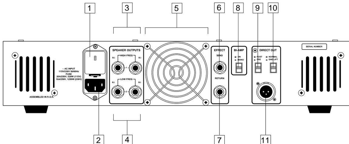
**1. Fuse sled** - This contains a fuse holder and shows the currently selected voltage rating for your Model 5000/7000. **Make sure the voltage rating is correctly set before powering up the amplifier!** Fuse ratings for the Model 5000 are: 15 amp for 115 VAC and 8 amp for 230 VAC. Fuse ratings for the Model 7000 are: 20 amp for 115 VAC and 10 amp for 230 VAC. For information on how to change the voltage rating, see Appendix C on page 14.
