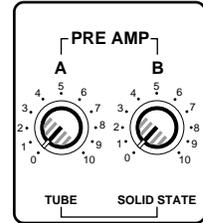
9. When you have settled on a Pre-Amp balance, the next step is to adjust the two Contour (bass and treble equalizer) controls to taste. For more information, see the “About Equalization” section on page 9 of this manual. When you get a great setting that complements your instrument and playing style, it’s a good idea to write it down for future use.
