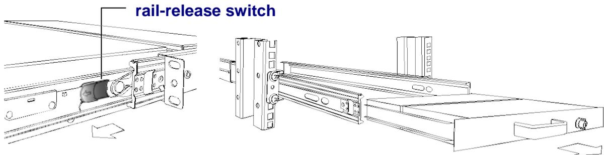
8. Push rail-lock switch on the rail and push rail back.(Both sides)
