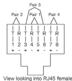
Figure 4-4. CAT5/5E/6 Straight Through UTP/STP Cable (8P8C)
