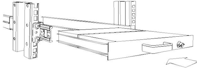
6. Unlock and pull rail-lock switch (left and right at the same time) then push console to the end.
