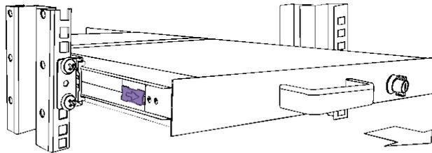
5. Pull rail-release switch and pull console out.(Both sides. Be careful when pull out console.)
