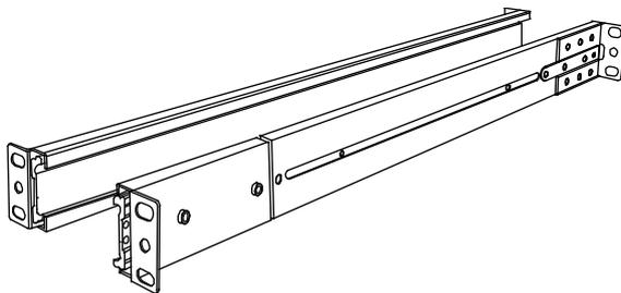
2. Long bracket x 2. (Needed for rack depth 828 ~ 1000mm)
