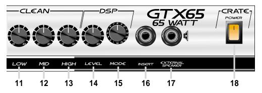
**16: INSERT:** Use this jack to connect an external effects device to the amplifier. Use a stereo 1/4" male Y connector: ring = send, tip = return, sleeve = ground. (Refer to the illustration at the bottom of page 5.)
