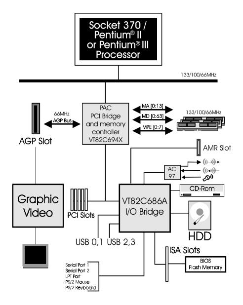
Figure 5: System Block Diagram
