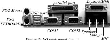
Figure 3: I/O back panel layout
