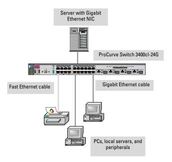
The Switch is designed to be used primarily as a desktop switch to which end nodes, printers and other peripherals, and servers are directly connected, as shown in the above illustration. Notice that the end node devices are connected to the switch by straight-through or crossover twisted-pair cables. Either cable type can be used because of the "IEEE Auto MDI/MDI-X" features on the Switch.
