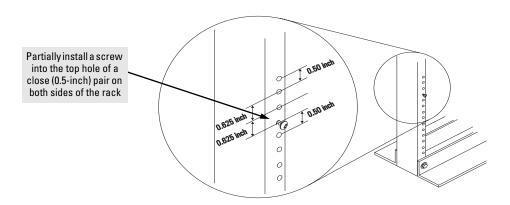
3. Place the switch in the rack and lower it so the notches in the bottom of the bracket slide onto the screws, then tighten these screws.
