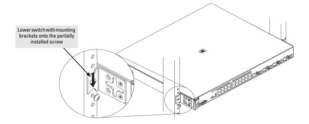
$\begin{tabular}{ll} 4. & In stall the other number $12$-$24 screw into the upper hole in each bracket. \\ & Tighten these screws. \\ \end{tabular}$
