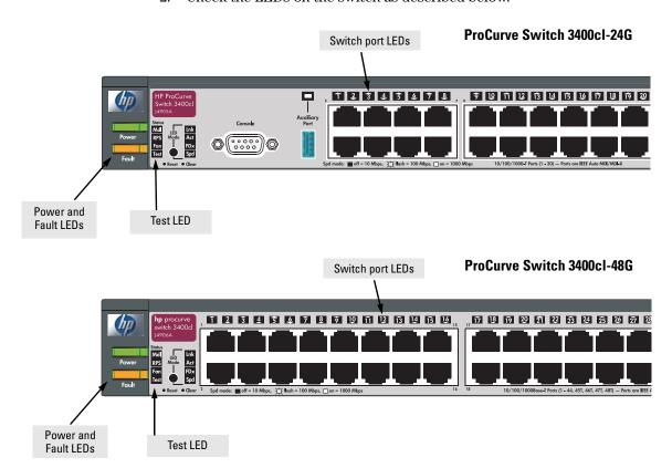
When the switch is powered on, it performs its diagnostic self test. Self test takes approximately 50 seconds to complete.
