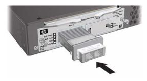
**b.** Push firmly until the gasket seats against the bulkhead.
