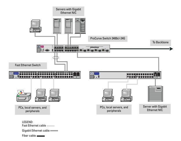
The Switch also works well as a segment switch. That is, with its high performance, it can be used for interconnecting network segments—simply connect the network hubs that form those segments to the switch, or you can also connect other switches.
