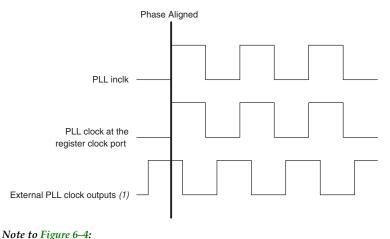
Figure 6–4. Phase Relationship Between PLL Clocks in Normal Mode
