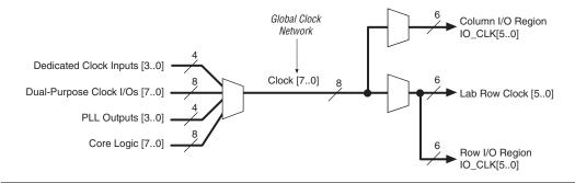
IOE clocks have horizontal (row) and vertical (column) block regions that are clocked by six I/O clock signals chosen from the eight global clock resources. Figure 6–20 shows the I/O clock regions.
