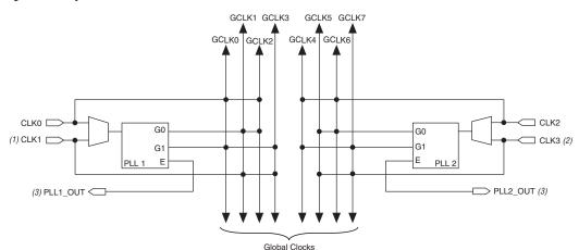
Figure 6-3. Cyclone PLL Clock Connections
