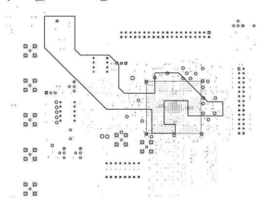
Figure 6–7.  $V_{CCINT}$  Plane Partitioned for  $V_{CCA}$  Island
