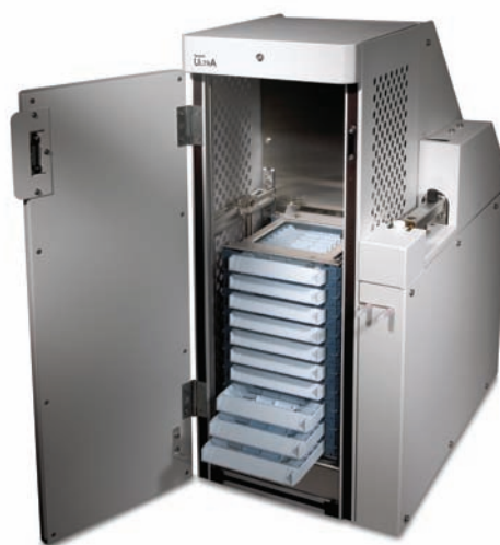
Series 2 ULTRA: 10 trays, each accommodating up to 10 capped tubes, shown here with '50:50' option for automating sample re-collection (SecureTD-Q)
