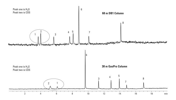
Chromatographic example two: Demonstrates hydrocarbon quenching by C3s and the solution strategy of chromatographic selectivity.
