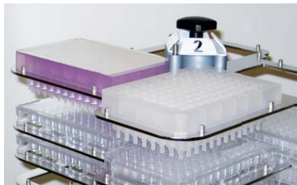
Figure 3: Cutouts in the shelves are suitable for holding filter plates.
