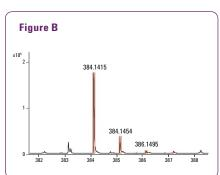
For pesticide analysis, the 6550 iFunnel 0-TOF demonstrated (Figure A) 10-fold sensitivity gain for a poor responding pesticide (fluazifop-butyl) in pepper matrix. Extracted ion chromatogram shows excellent detection (S/N 1200) on 10 ppb fluazifop-butyl and (Figure B) confident compound identification of fluazifop-butyl with an excellent library match score of 98 based on a mass error of only 0.5 ppm and correct fit of isotope abundance and spacing.
