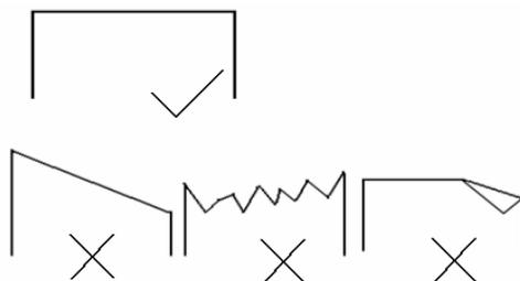
Make sure that the heat sensitive side of paper faces the print head and the rolling direction of paper meets the requirements.
