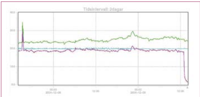
Since the installation of the ACS 1000 variable speed drives and a new control system, the differential pressure has been controlled automatically, which resulted in a more accurate and stable pressure in the district heating piping system.
