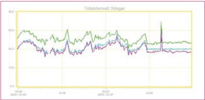
The manual control of the differential pressure in the district heating piping system resulted in considerable fluctuations.
