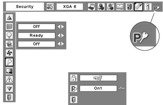
When the projector is locked with a PIN code, the PIN code lock symbol appears on the menu bar.
