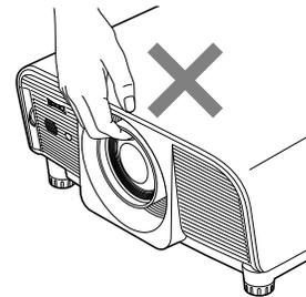
Do not hold the lens and the peripheral part.
