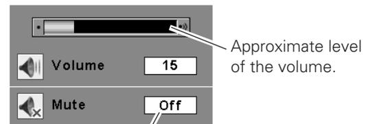
Press the MUTE button to set the Mute function On or Off. The dialog box disappears after 4 seconds.
