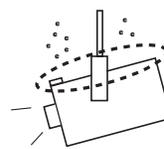
When hanging the projector from the ceiling, clean air intake vents, filters, or top of the projector periodically with a vacuum cleaner. If you leave the projector unclean for a long time, the cooling fans can be clogged with dust, and it may cause a breakdown or a disaster.
