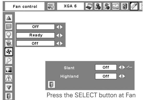
Press the SELECT button at Fan control and this dialog box appears. Use the Point ▲▼ buttons to choose Slant or Highland. Use the Point ◀▶ buttons to switch between the options.
