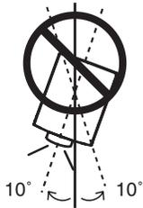
In downward projection, do not tilt the projector over 10 degrees right and left.
