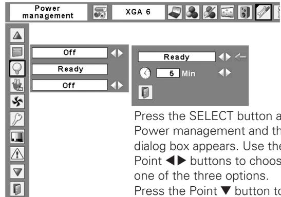
Press the SELECT button at Power management and this dialog box appears. Use the Point ◀▶ buttons to choose one of the three options. Press the Point ▼ button to select the timer, and then use the Point ◀▶ buttons to set timer.
