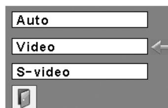
\* If the projector cannot reproduce proper video image, select a system manually (see "Video System Selection" on page 36).
