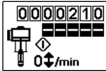
2. While in Prime/Flush mode, runaway protection is disabled and the batch totalizer (BT) will not count.
