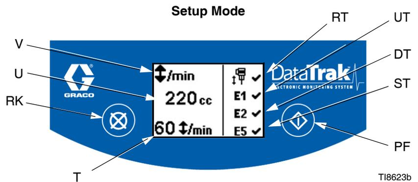
FIG. 3. DataTrak Controls and Indicators
