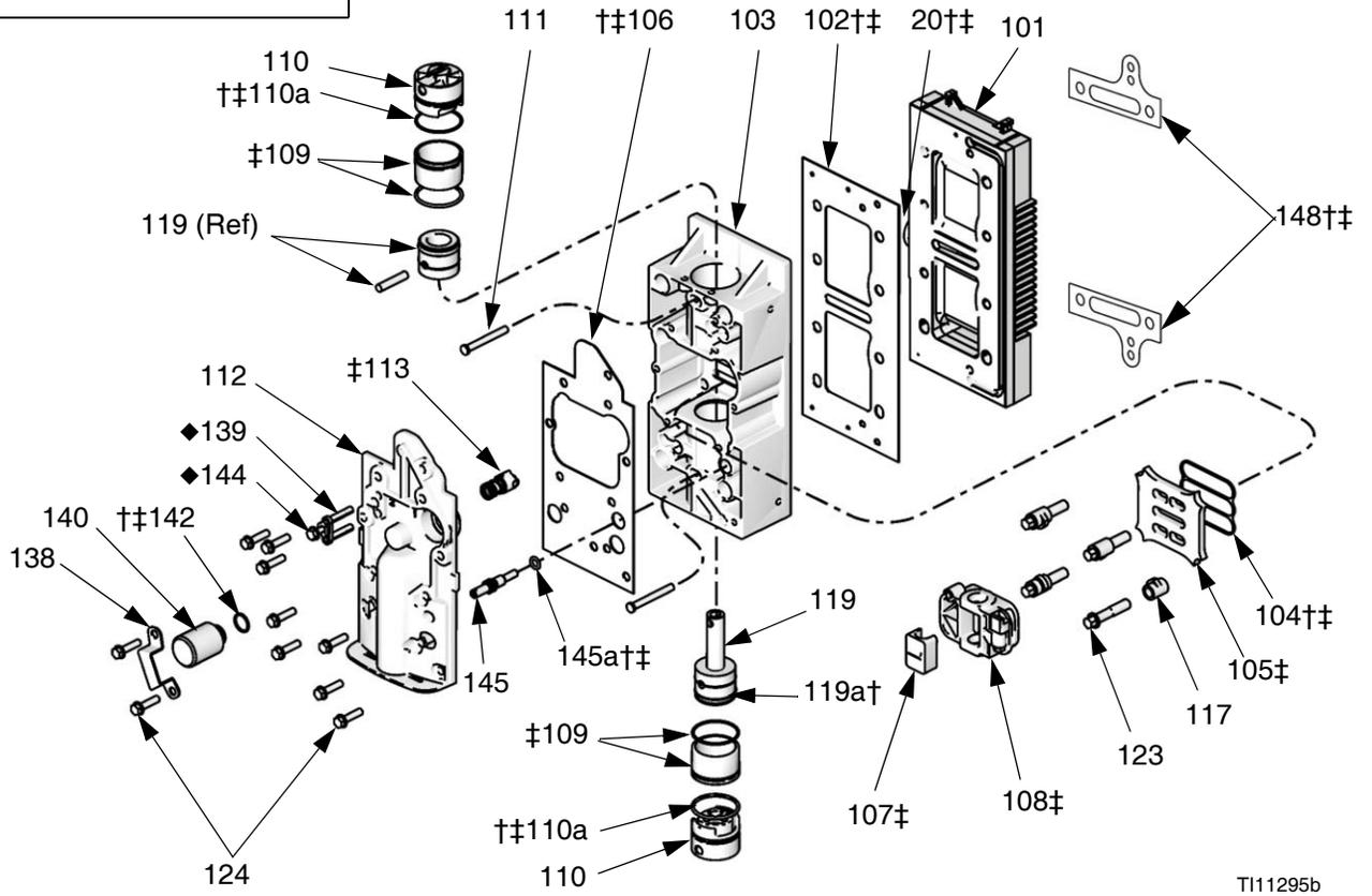
**Part NXT107 Bare Air Valve****Part NXT108 Air Valve with DataTrak Module (shown)****Part NXT109 Air Valve with Junction Box Housing**
