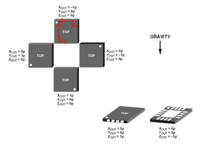
Figure 3. Output Response vs. Orientation
