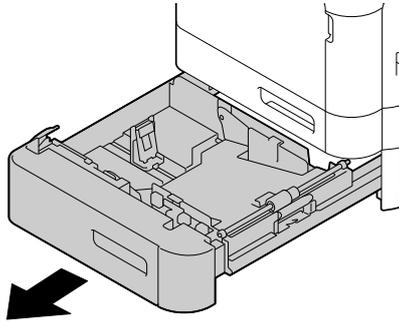
2 Press the flip-top plate down until it is locked.
