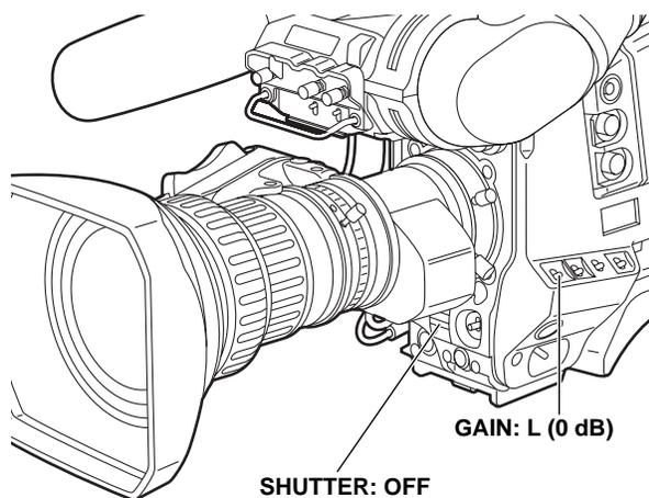
**3** If the lens is provided with an extender, disengage the extender function.
