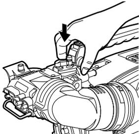
**4** Tighten the stopper screw firmly.
