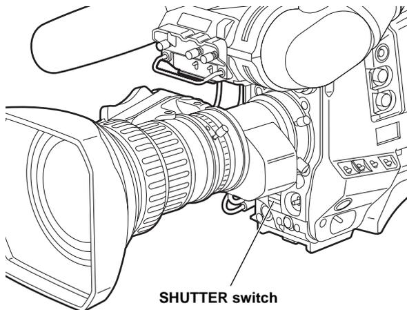
**3** Press the SHUTTER switch to the SEL position again, and repeat this until the desired mode or speed is displayed. When all the modes and speeds are displayed, the display will change in the sequence shown below. When the required shutter speed and mode have been assigned beforehand, only the assigned speed or mode will be displayed.
