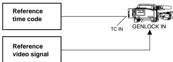
The built-in time code generator is now locked to the reference time code.
