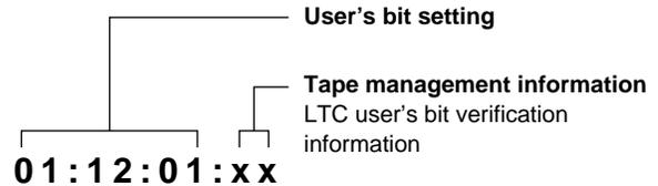
To verify the VITC user's bit, set the DISPLAY switch to UB, and hold down the HOLD button. While the HOLD button is held down, the VITC user's bit information appears on the counter display.
