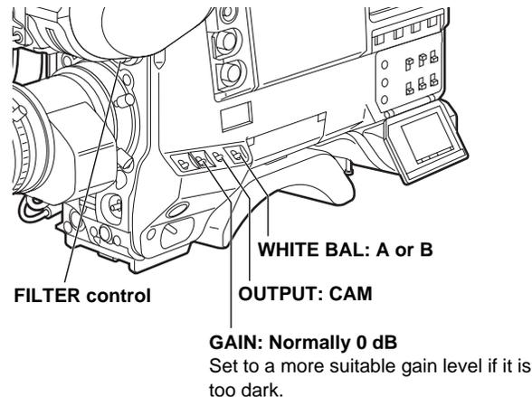
When the GAIN and WHITE BAL switch settings are changed, messages advising the user of the set positions appear on the setting change message display of the viewfinder screen. (However, this happens only when “3” has been set as the display mode.)
