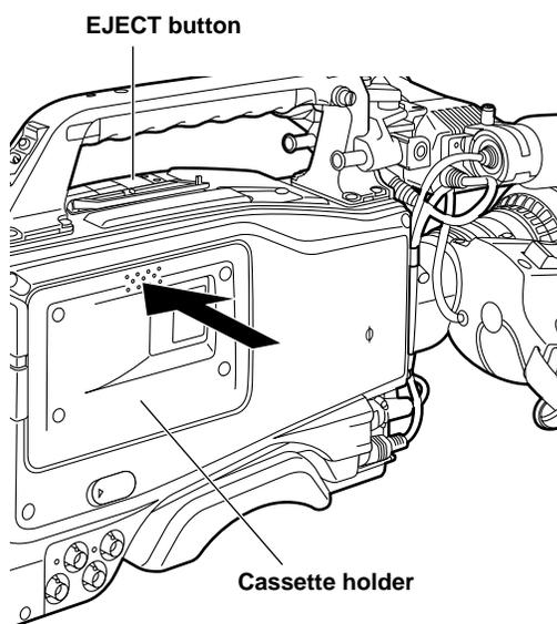
**3** Insert the cassette tape and press the part marked with the arrow to close the cassette holder securely.
