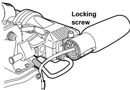
**3** Connect the microphone's connecting cable to the MIC IN jack on the camera.
