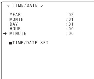
**3** Turn the JOG dial button to change the setting, and press the JOG dial button to enter the setting.
