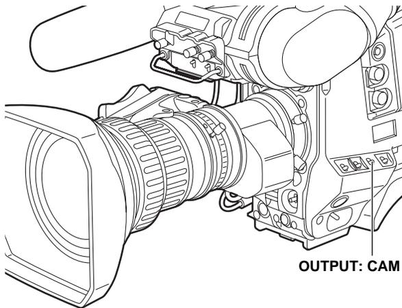
**2** Set the AUTO W/B BAL switch to the ABB position, and then release it. The switch returns to the center, and the adjustment is performed.
