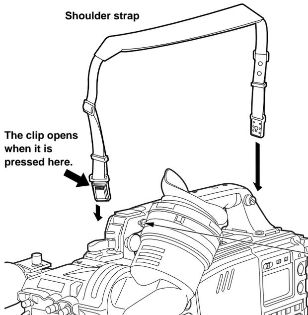
To detach the shoulder strap, open the clips on the mounting parts and detach.
