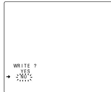
**7** Turn the JOG dial button to move the arrow (cursor) to YES, and press the JOG dial button. The data settings are saved in the scene file area of the camera's memory.
