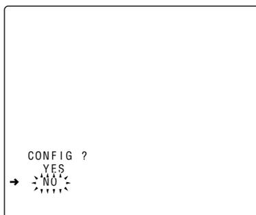
**4** To proceed with the formatting of the setup card, turn the JOG dial button to move the arrow (cursor) to YES, and press the JOG dial button. When the formatting of the card is completed, the following message appears.
