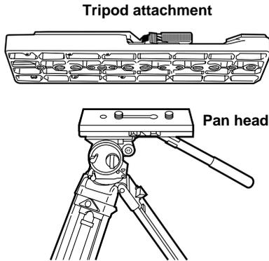
**2** Attach the camera to the tripod attachment. Slide the camera toward the front along the grooves until it clicks into place.
