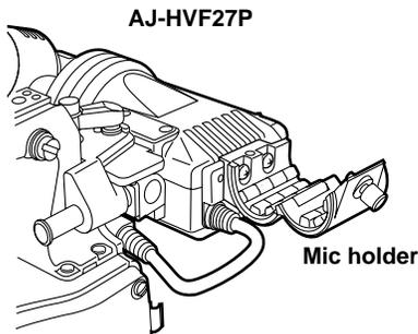
**2** Attach the microphone, and tighten the locking screw.
