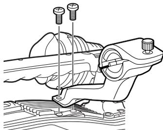
**3** Attach the microphone to the mic holder, and tighten the locking screw.
