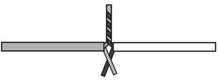
3. Lay upper twisted pair of wires over right wire as shown. Bring lower twisted pair of wires up to meet the left wire as shown.
