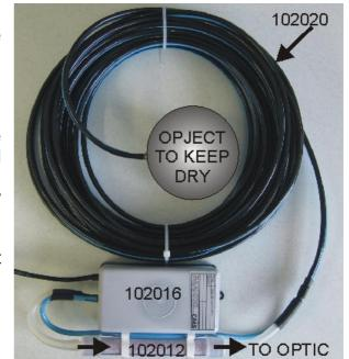
The dry air pump re-circulates air through the connected elements. This air is also passed through a drying tube. The desiccant changes colour when saturated and should be replaced. Connect the hose with about 6mm inner diameter to the marked connectors on the right side.
