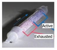
Indicating DRIERITE in this plastic unit dries air and gases for small scale laboratory applications. A rubber hose connection provides an immediate flow of dry gas.
