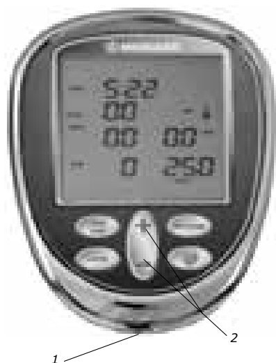
Fig: Workload adjustment and connections 1) USB 2) Workload adjustment (+/-)
