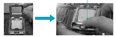
7. Lower the lever and lock it to the load plate, then the CPU is locked completely.
