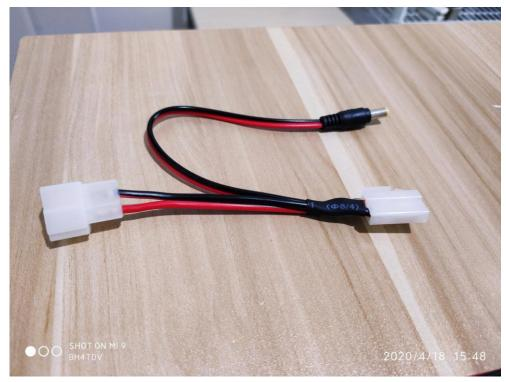
51WG5 comes with a dedicated power cord. Connected in series with the power cord of the radio, split out a DC plug to supply power .
