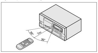
If the remote control sensor window is in a position where it receives strong light such as sunlight or fluorescent light, control may not be possible.
