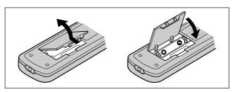
Open the lid of the battery compartment on the rear of the remote control unit, and insert the batteries, taking care to align the (+) and opolarities correctly.
