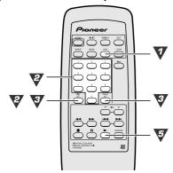
Operation example) Programming disc 2, track 7 as step 1, and disc 5, track 3 as step 2.
