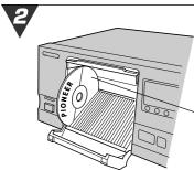
Load the disc into the rack with the label side (printed surface) facing to the right.
